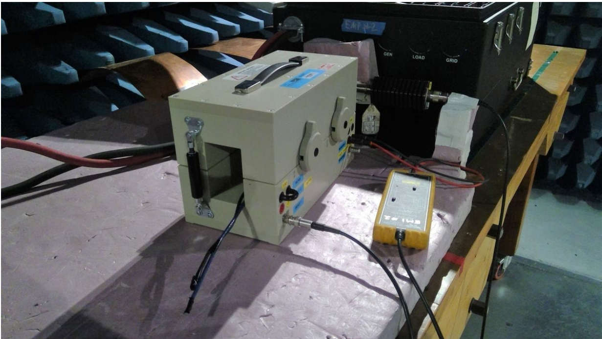
6 CS117 Active Load Testing
