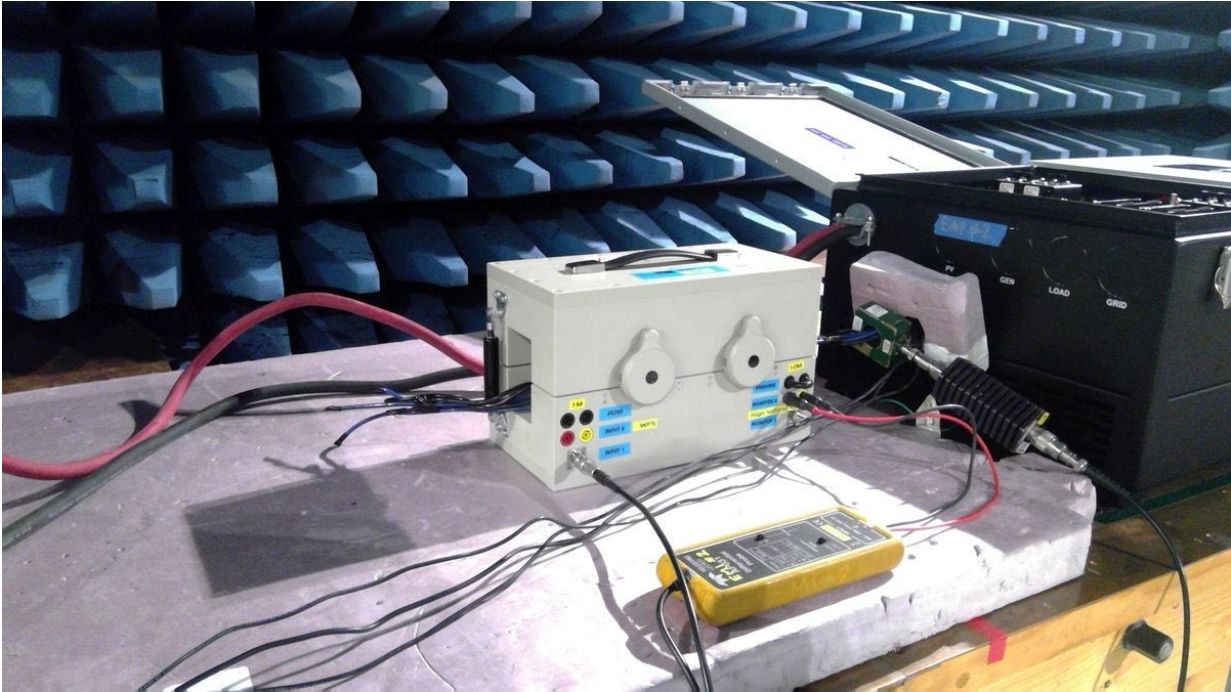
5 CS117 Active Load Bundle Testing
