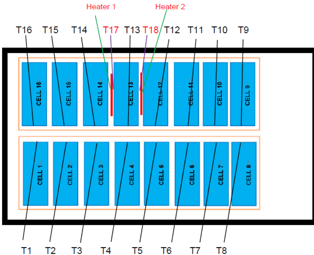
Figure 5. Schematic illustration of film heaters and thermocouple locations in initial module (T1 to T18 means thermocouples T1 to T18. H1, H2 means Film heater 1 and 2. View from top.).
