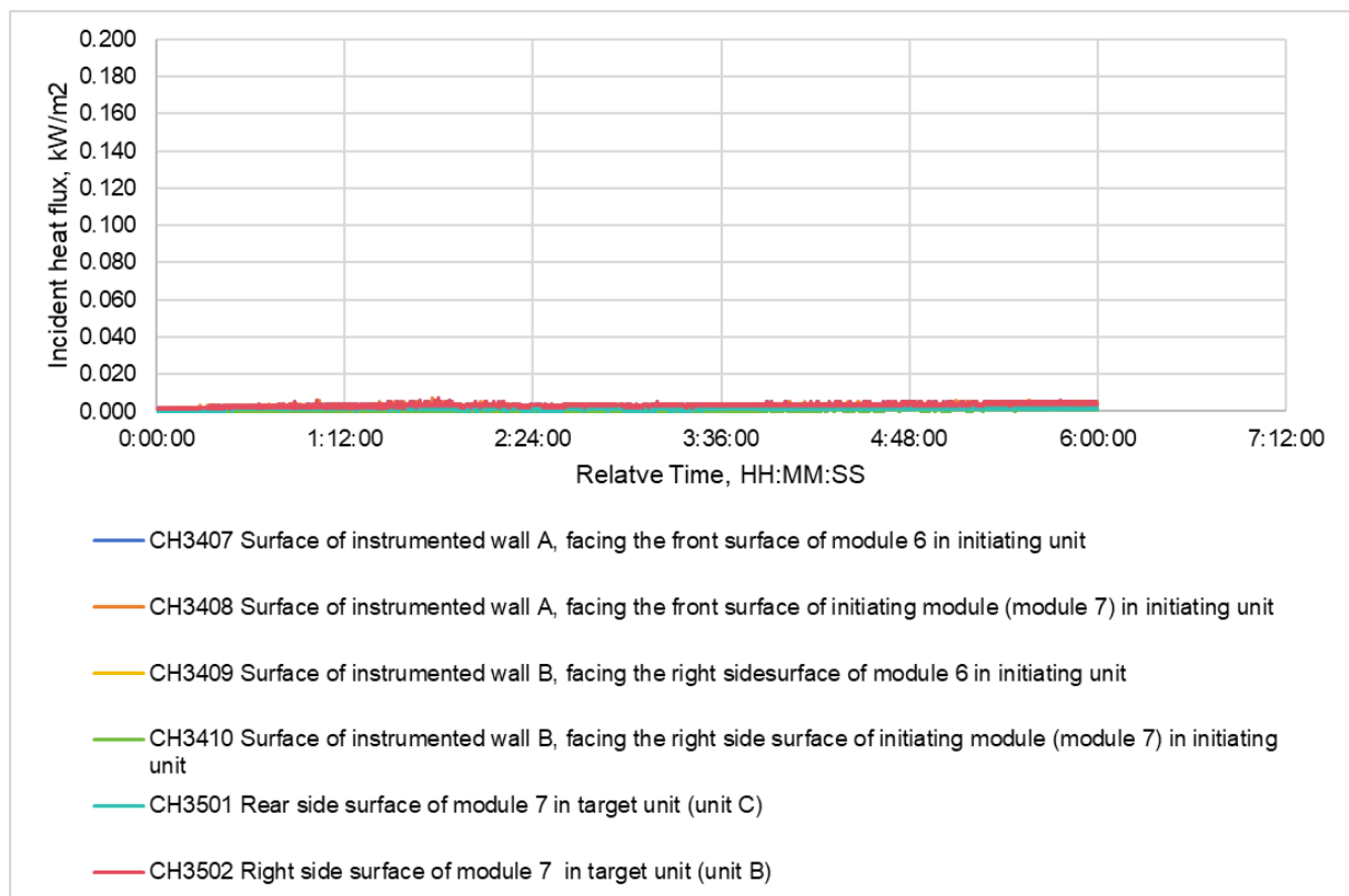
Figure 15. Incident heat flux on instrumented wall surfaces and target units
